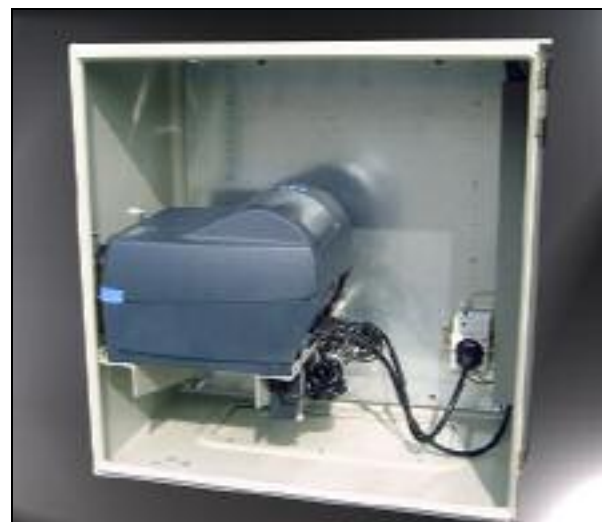
Printer in over pressurized panel
